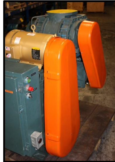
Model 1736 is a combination of a Stokes 212 Pump and a Stokes 607 Booster Pump Assembly
