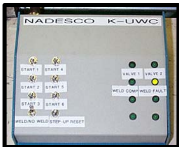
Dedicated Control Panel
